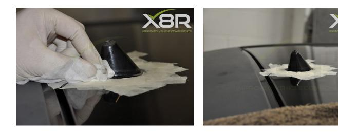
Step 5: Fitment of new seal Slide the new seal over and onto the aerial, with a blunt item push the inner lip into the recess underneath the aerial.
