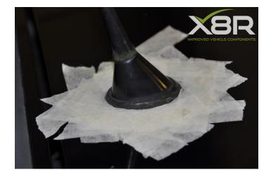
Step 2: Loosening seal from aerial Using a sharp blade, carefully put a slit into the seal, then pry out the damaged seal from underneath the aerial.
