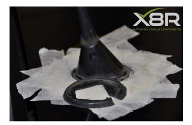
Step 3: Unscrew the aerial At this point it would be advisable to unscrew the aerial as it can obstruct the fitment of the seal.
