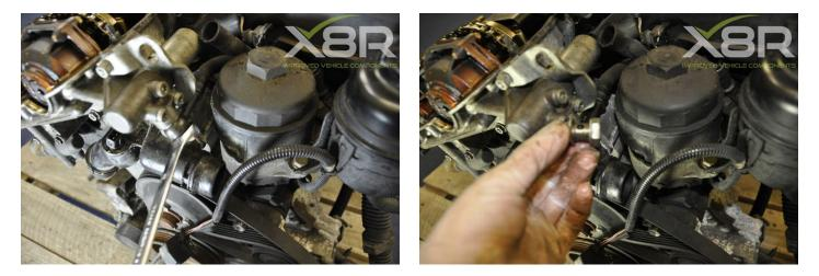
Step 8: Remove engine lift bracket • Remove engine lift bracket from Vanos unit using 11mm socket top bolt and 13mm socket bottom bolt. Rotate bracket bottom to top then remove
