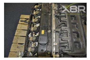
Step 2: Remove valve cover vent hose
